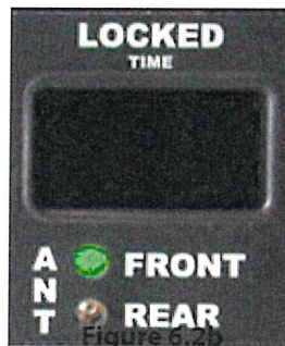
Figure 6.2b When the FRONT light illuminates, the FRONT antenna is transmitting.
