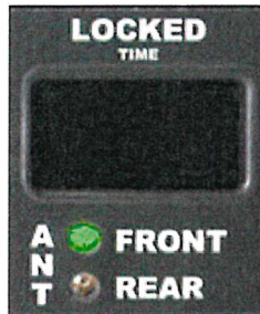
Figure 3.2.2.4b Antenna lights showing front antenna is active
